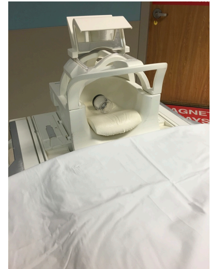
Figure 6. Phantom Lipid in head coil of 1.5T MRI
