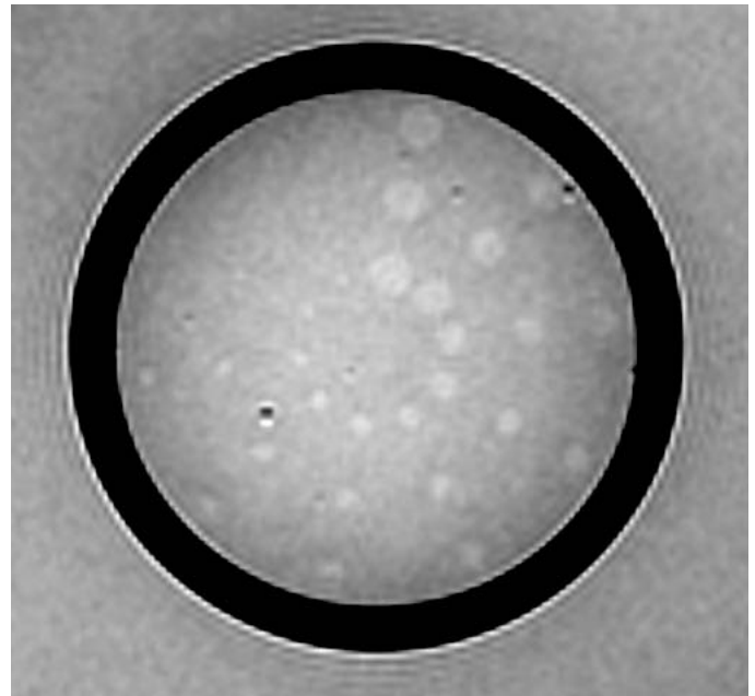
Figure 19: Image of slice 8, magnified and cropped, showing the circle of low-contrast objects. This image would be scored as showing 9 spokes. The ninth spoke may be difficult to see on the printed image.
